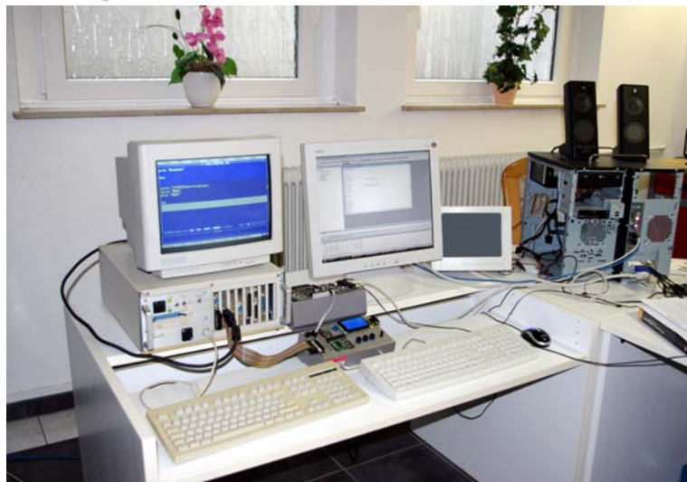
Emulation of the parallel port by means of an Atmel AVR microcontroller. Two different units are provided. One is the host; the other emulates a peripheral device. Here the prototype of the peripheral device emulator is shown. The successors will be based on the microcontroller modules depicted above.
