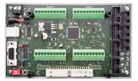
The photos show the first prototype (V1). Further development led to omitting the RS-232 signalization, reducing the number of jumpers to two, and changing the USB connector to mini-B.
